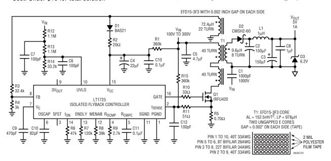
100V<sub>IN</sub> to 300V<sub>IN</sub>, 5V<sub>OUT</sub> at 1A Isolated Flyback Power Supply
